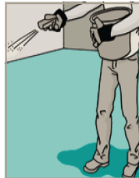
Broadcast the coating with quartz sand before it has completely cured.
