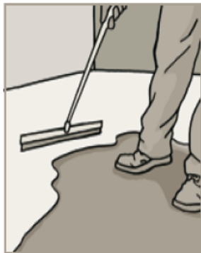
Apply primer to the clean, dry substrate using a squeegee and roller.
